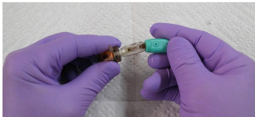
Figure 4 – Installation of the skin by sliding onto the core
